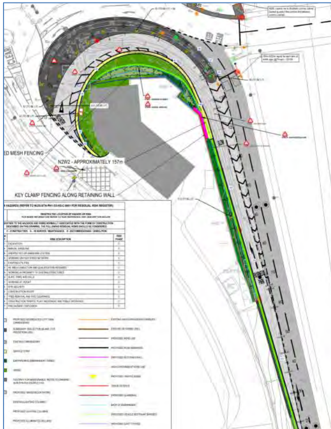
Figure 30: Stantec Design of Potential Left-turn Slip Lane from A404 NB Off-slip to Parkway
