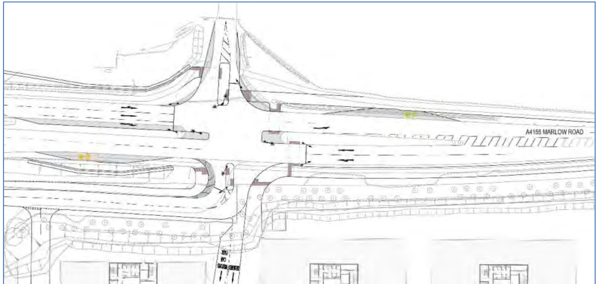
Figure 32: AECOM Option 1 Conceptual Design for Proposed A4155 Marlow Road / Site Access / Pump Lane South Signal-Controlled Junction
