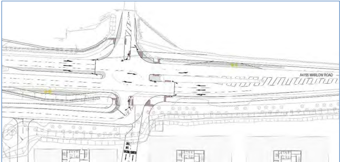
Figure 34: AECOM Option 2 Conceptual Design for Proposed A4155 Marlow Road / Site Access / Pump Lane South Signal-Controlled Junction
