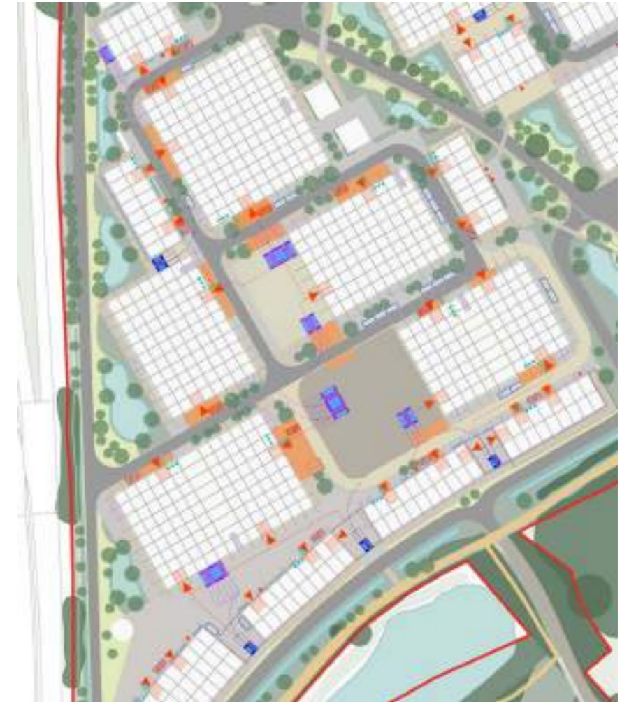
Figure 6.74 West Cluster Indicative Operational Plan - Deconstruction Stage
